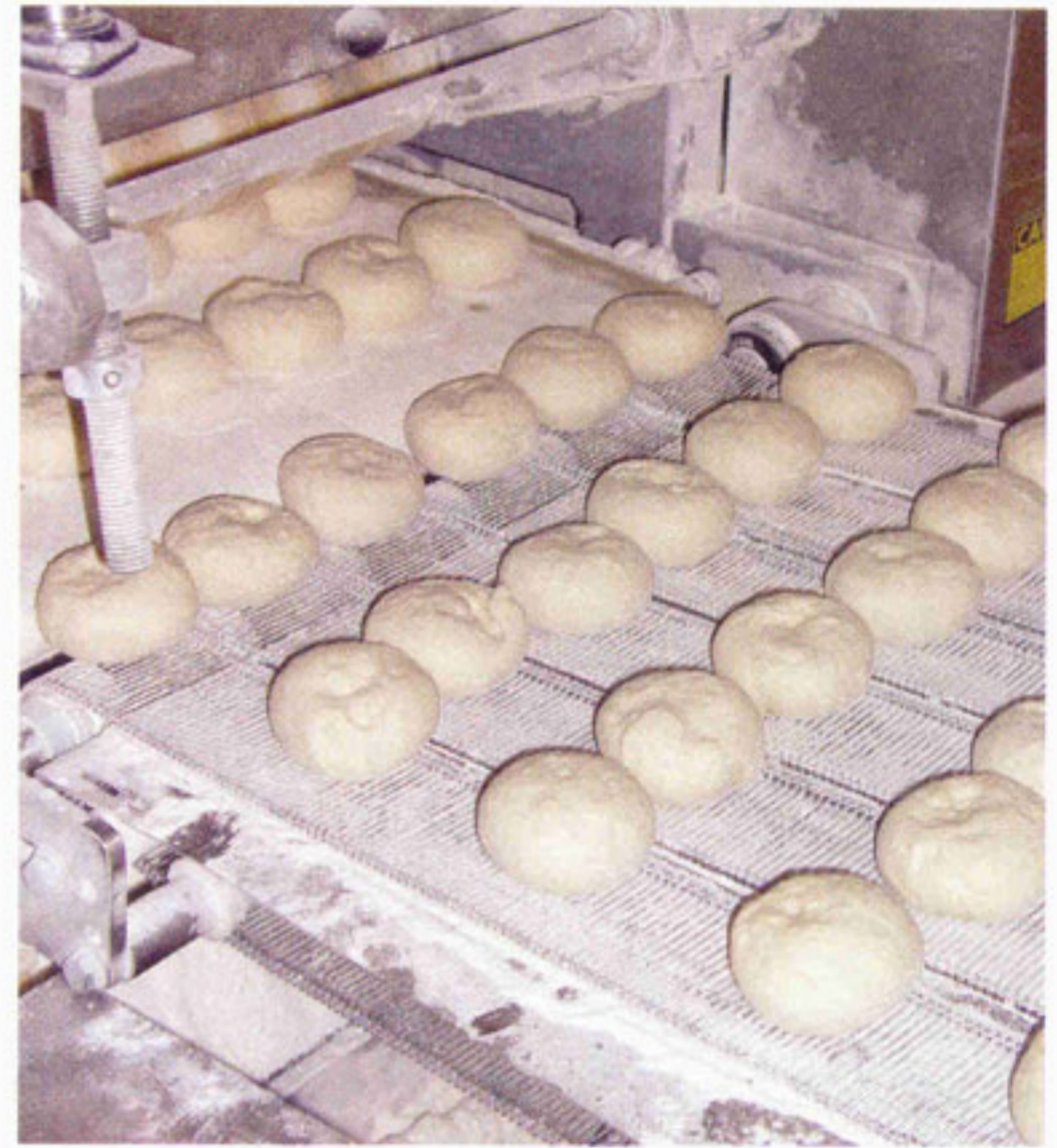
▲ Roll pieces proceed from the automated roll line's divider into its intermediate proofer.
